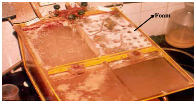
Fig. 2. An image of foaming in the condition of PA concentration of 500 mg/l and HRT of 6 h.
